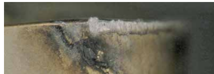
Cutting Edge Conditions Comparison - after 40 min machining - (Internal Evaluation)
