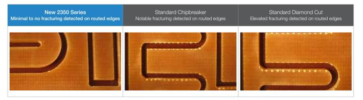
Users of the Series 2350 routers report 70% to 94% reduced fracturing when comparing to other router designs. Please contact a Kyocera Precision Tools field engineer for process assistance.
